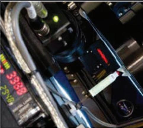
Eight camera inspection system for case defect detection
